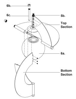
Attach bottom section to top section with screws (6a), followed by screw cover (6c) and secure with finial (6b) by threading clockwise
